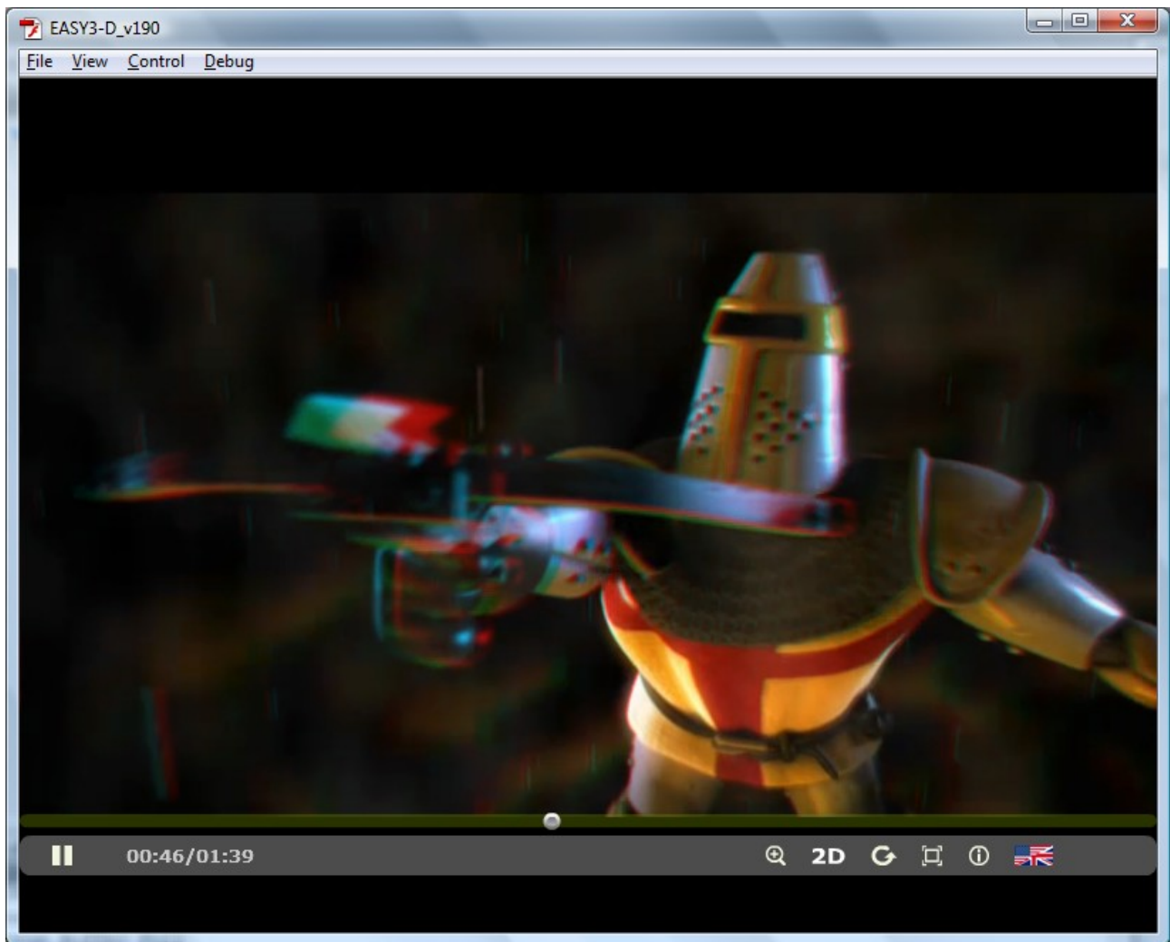
Fig. 3: a screen view of a 3-D movie encoded in red/cyan anaglyph on-the-fly (frame by frame in real time) by EasyGO 3-D Player
